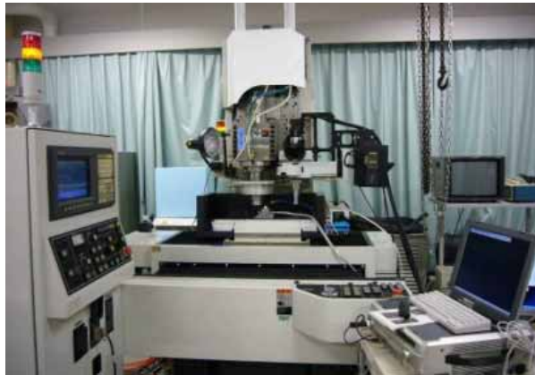
Automatic serial-sectioning device
