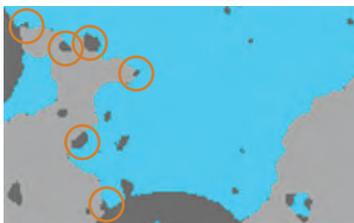
**Fig. 3.** Segmentation showing the Zener pinning mechanism with a low contrast boundary.
