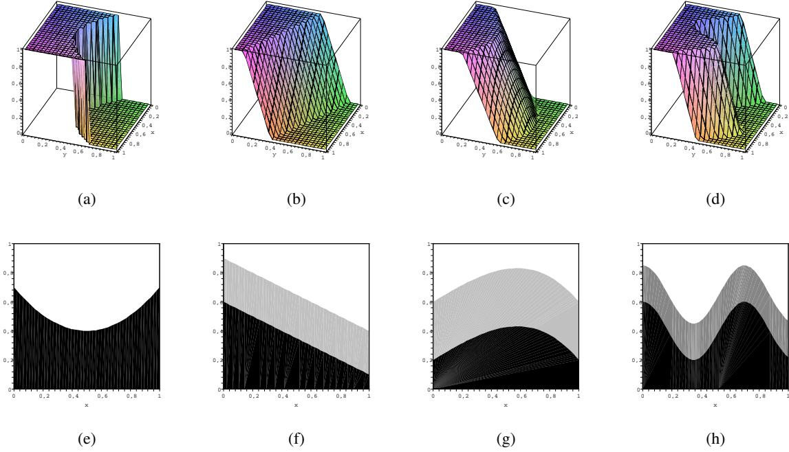
Fig. 3. Examples of smoothlets: (a)  $r = 0$ ,  $b(x) = 1.2x^2 - 1.2x + 0.7$ , (b)  $r = 0.3$ ,  $b(x) = -0.5x + 0.6$ , (c)  $r = 0.4$ ,  $b(x) = -0.6x^3 + 0.6x + 0.2$ , (d)  $r = 0.25$ ,  $b(x) = 0.2 \cos(9x) + 0.4$ ; and (e)–(h) their corresponding projections, colors: black, white — areas of constant part, grey — area of linear part.
