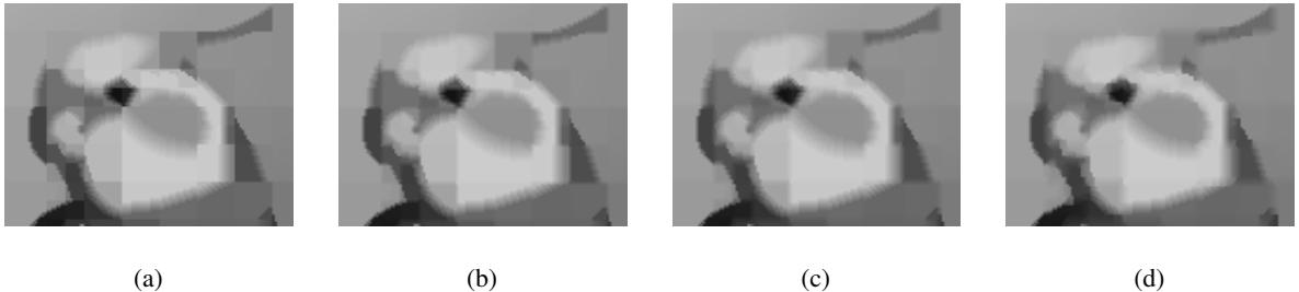
Fig. 13. Results of postprocessing for zoomed image “Bird,” (a) no postprocessing, PSNR=29.837 dB, (b) 1-pixel averaging, PSNR=29.957 dB (c) 2-pixel averaging, PSNR=30.272 dB (d) 4-pixel averaging, PSNR=29.838 dB.
