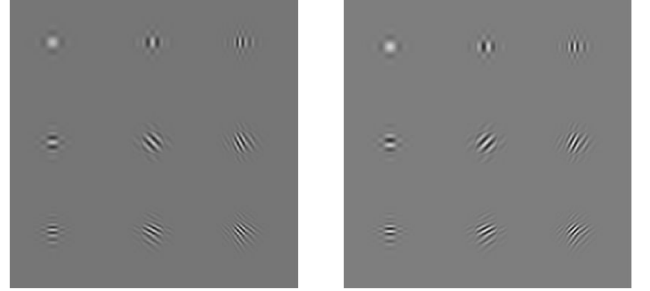
Figure 3: Bidimensional 3-band dual-tree wavelets: (Left) negatively oriented scaling function and wavelets; (Right) positively oriented counterparts.
