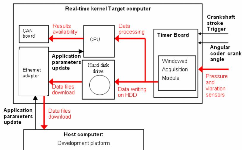
**Figure 1: Combustion Analysis Platform hardware architecture diagram.**
