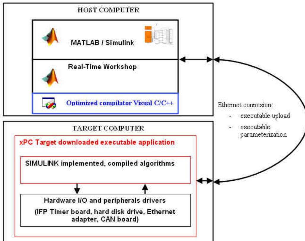
**Figure 2: Fast prototyping software architecture diagram.**
