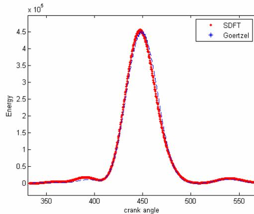
**Figure 7: Comparison of the spectral component energy versus angle determined with Goertzel and SDFT algorithms.**
