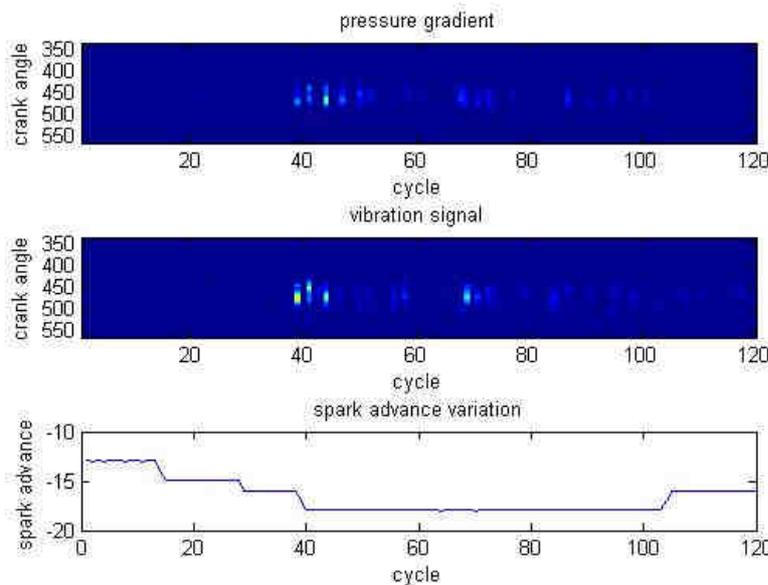
**Figure 8: Real time knock analysis of the first test at 1500 rpm and 6 bars IMEP (top: results from the application of the proposed methodology applied to the pressure signal, middle: results from the same methodology applied to the vibration signal, bottom: spark advance).**
