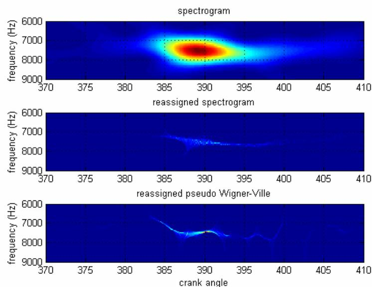
**Figure 5: Spectrogram (top), reassigned spectrogram (middle), reassigned pseudo Wigner-Ville distribution (bottom).**
