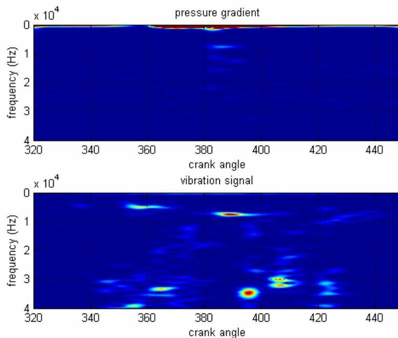
**Figure 4: Pressure gradient and vibration signal spectrograms.**
