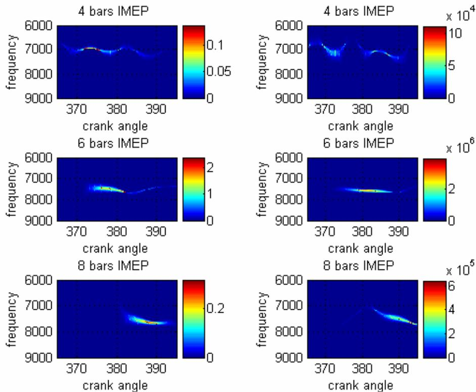
**Figure 6: Knock frequency variation due to load increase (pressure on the left and vibration signal on the right).**
