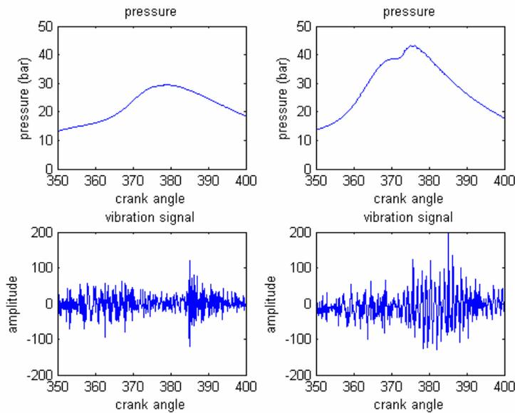
**Figure 3 : Pressure and vibration signals in non-knocking and knocking condition.**
