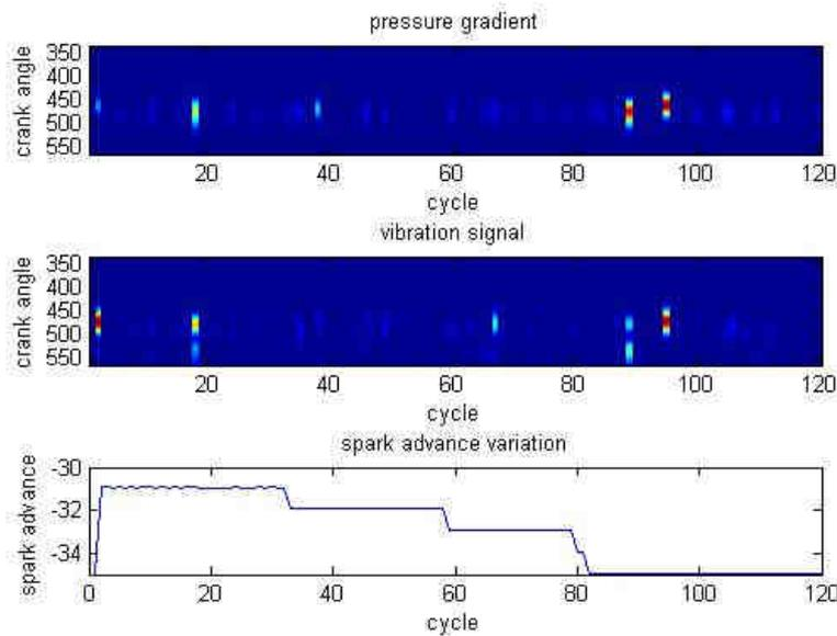
**Figure 9: Real time knock analysis of the second test at 3000 rpm and 6 bars IMEP (top: results from the application of the proposed methodology applied to the pressure signal, middle: results from the same methodology applied to the vibration signal, bottom: spark advance).**
